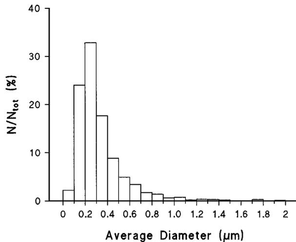
Figure 13 Distribution of particle sizes evaluated by computerised image analysis from several micrographs as Fig. 12.
