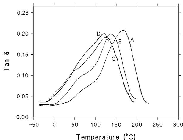
Figure 14 Dynamic-mechanical spectra in terms of  $\tan \delta$  in the temperature range  $-50$  to  $300^\circ\text{C}$ . a) Plain UP resin; b) 80/20 composition; c) 70/30 composition; 60/40 composition.
