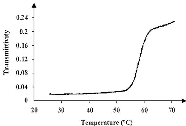
Figure 17 Transmittivity versus temperature curves in the range 20°C–80°C for the 60/40 composition.
