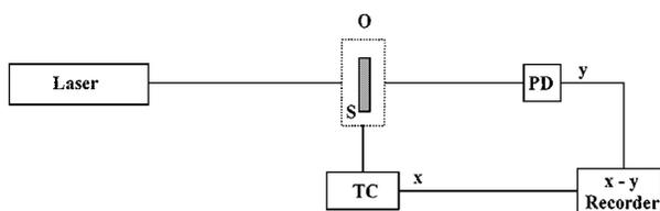
Figure 1 Experimental set-up for thermo-optical analysis. O: oven; S: sample; TC: temperature control; PD: photodiode.
