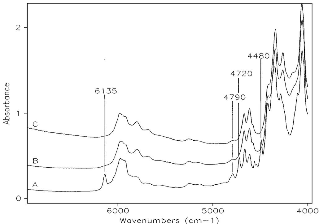
Figure 5 FT-NIR spectra in the 7000–4000  $\text{cm}^{-1}$  of the 70/30 PDLC formulation prior to curing (trace A); the same sample after curing; the 60/40 formulation after curing.
