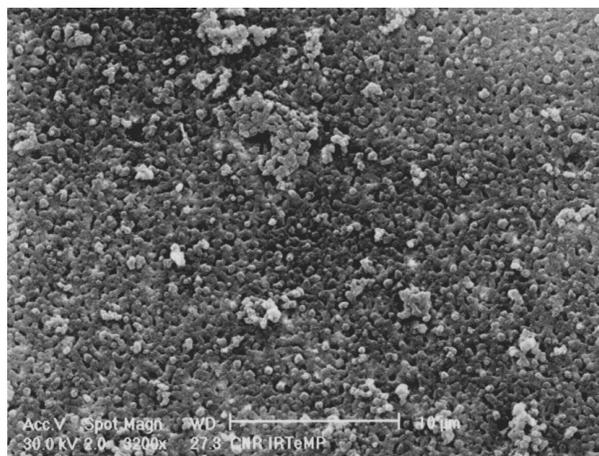
Figure 12 High magnification SEM micrograph of the etched surface of the 60/40 PDLC composition after curing.
