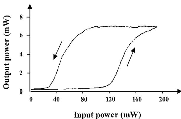
Figure 18 Output power as a function of the input power near the transition temperature for the vertical component of the light polarisation. Measurement taken on the 60/40 composition.
