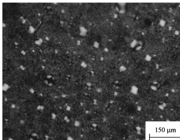
Figure 9 Optical micrograph taken at ambient temperature under polarised light of the 60/40 PDLC composition after curing.
