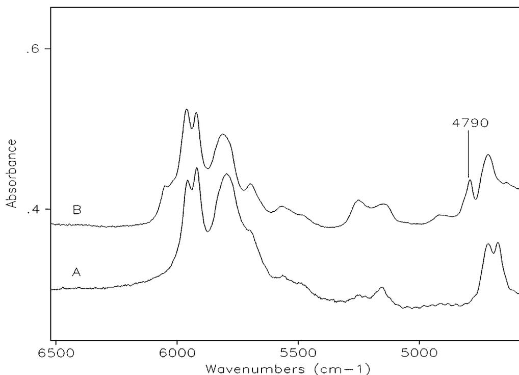
Figure 4 FT-NIR spectra of dibutylsuccinate (trace A) and dibutylfumarate (trace B) in the frequency range 6500–4500  $\text{cm}^{-1}$ .
