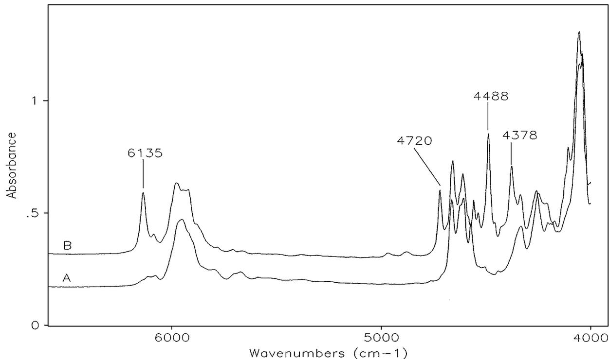
Figure 3 FT-NIR spectra of polystyrene (trace A) and styrene (trace B) in the frequency range 6500–4000  $\text{cm}^{-1}$ .
