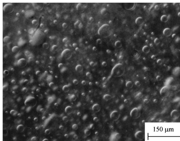
Figure 8 Optical micrograph taken at 70°C under unpolarised light of the 60/40 PDLC composition before curing.
