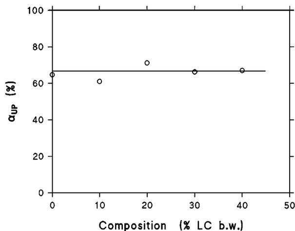
Figure 6 Conversion of the fumaric double bonds of the polyester after the photo-polymerisation process as a function of the LC content in the PDLC system.
