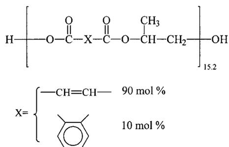
The formulation used in the present contribution contained 35 wt % of styrene as co-reactive monomer; therefore the initial molar ratio between styrene and polyester unsaturations was 1.1. The molecular structure of the cured network is schematically represented below:
