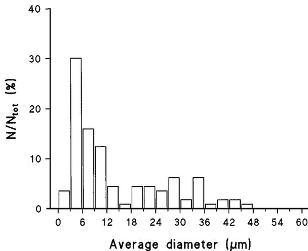
Figure 11 Distribution of particle sizes evaluated by computerised image analysis from several micrographs as Fig. 10.
