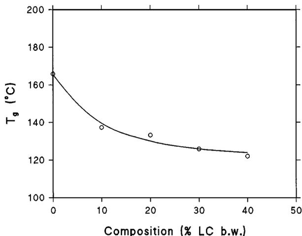
Figure 15 Glass transition,  $T_g$ , as a function of the LC content in the PDLC system.
