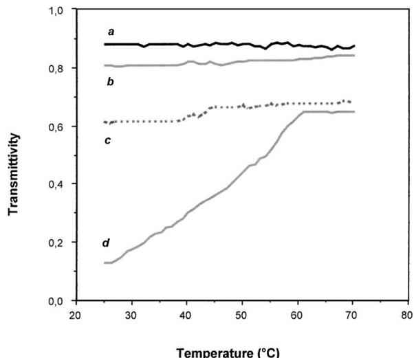
Figure 16 Transmittivity versus temperature curves in the range 20–80°C for a) plain UP resin; b) 90/10 composition; c) 80/20 composition; d) 70/30 composition.
