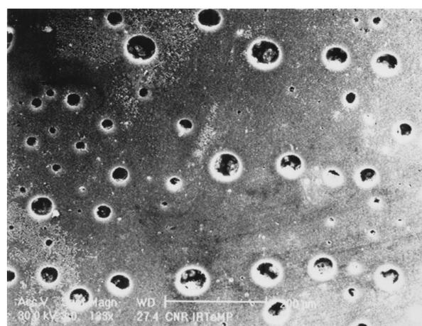
Figure 10 Low magnification SEM micrograph of the etched surface of the 60/40 PDLC composition after curing.
