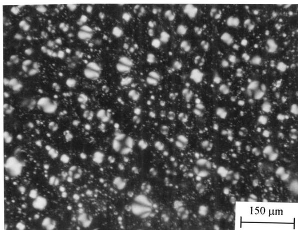
Figure 7 Optical micrograph taken at ambient temperature under polarised light of the 60/40 PDLC composition before curing.
